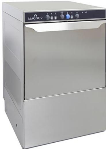
Partial double skinned body; stainless steel arms, injectors and body; preformed wash tank; preformed rack guides; double panel door; automatic water supply; safety device on the door; rinsing with hot water through thermostop system; built-in rinse aid dispenser; adjustable thermostat for tank and boiler; electromechanical controls; extractable control panel; integrated water suction group from the tank and drain for total drainage of the washing circuit (gravity drain); anti-backflow valve.
