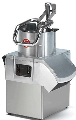
Large production head with lateral blade, which distributes the product inside the inlet, and handles entire products such as cabbage. The core drill (included) can also be used to achieve the same purpose.
